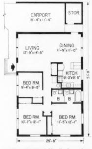
4-INCH MODULE of Morell plan reduces cutting of SCR brick to virtually nothing. Transite ducts in slab supply forced air.
