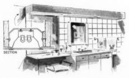
WALL-LENGTH soffit uses 3 commercially available units, two 40-Watt, 48" units in each. Note side brackets.
