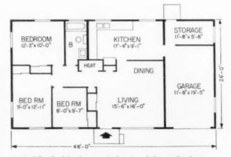
**PLAN** of Lauderdale shows typical traits of the one-level prefab: entrance at corner of living room, car area with storage and entrance to kitchen, closet sliders, flexible layout.
