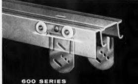
The Accepted Standard of Quality Satin finish aluminum track with built-in apron. Adjustable hangers. Nylon wheels with oiled-for-life bronze bearings. Only 1" headroom required.
