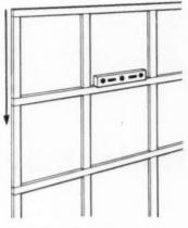
1 FURRING the wall. Check for plumb. Apply shims where needed, and insulation or moisture barrier to outside wall, before strips. Furr horizontally around room, then let in the vertical members 16" o.c.
