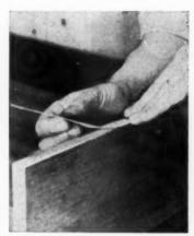
5 TREATING EDGE. Use hardwood strips or the new wood "tape" now available. First remove protective paper layer, then smooth on the wood tape as shown in photo, then bond to the edge with a warm iron.
