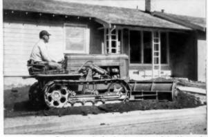
A great outfit for landscapers and builders—the John Deere "420" Crawler (with approximately 25 drawbar horsepower) and John Deere 6-foot dozer blade. So compact, it maneuvers within a one-car garage!
