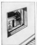
Build sleeve and frame into wall during construction. Opening is about 27" wide, 23" high. More through-the-wall units can be added later.
