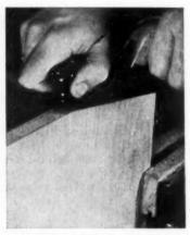
PLANING. Hold the plane in angled position as it runs along the plywood edge. Never run plane off the end of the edge. Instead, turn plane around and begin at that end to level up the cut.
