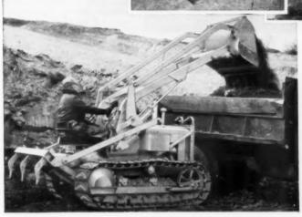
John Deere Crawler and Heavy-Duty Industrial Loader-Scarifier. Just the outlit for low-cost excavating, leveling, dirt moving, and similar jobs.
