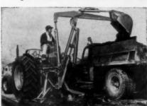
F. M. D. Tractor and Digger cuts costs of laterals, footings, service lines. Fast, positive hydraulic control. Fordson Major Diesel equipped with both rear-mounted backhoe and front-mounted loader makes an efficient, low-cost unit for excavating, loading, backfilling.
