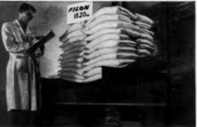
FILON MAS MUCH HIGHER LOAD CAPACITY THAN REQUIRED BY STANDARDS OF THE INDUSTRY. Shown above is a 26" wide FILON type 250 panel over a 4" span supporting a static load of 1820 lbs.—equivalent to 210 lbs. per sq. ft. Compare this with the 100 lbs. per sq. ft. required by industry standards.
