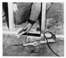
FOUR MINUTES to cut warm air duct opening (including 2x4 plate and direct cut into floor without starting hole) with B.C.S. Super Saw. Instant removal of saw from drill is made possible by a patented type of lug drive that provides a positive connection between the saw and the ½" electric drill. Circle No. 10009 on reply card.
