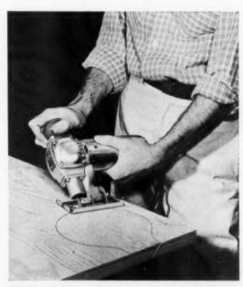
**BEVEL CUTS** on either side up to 45° is feature of Black & Decker jig saw No. 11. It has full one inch stroke; 2" depth at 90°, 1% at 45°. Shoe adjusts to any angle. The weight of the Heavy Duty jig saw is 6 lb. A metal-cutting blade and three high speed wood cutting blades are included. **Circle No. 10012 on reply card, p. 134.**
