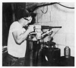
POWER HAMMER, under 13 lb., drills holes up to 11/8" diameter in toughest materials, Spring floated piston, neoprene mounted nozzle, induction hardened helical gears are featured in the Remington Rand H54U. It delivers up to 2300 blows per minute. The crank assembly is counterbalanced. Switch is sealed against dirt. Circle No. 10007.
