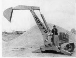
HYDRAULICALLY ACTUATED OUTRIGGERS are now built-in to this Hopto digger, Model 190 SPC-55. Operator can control each stabilizer individually for leveling machine on uneven terrain. Model has enclosed type boom and five-inch 1.D. cylinders on hoist, crowd and bucket-actuating equipment. Digging depth of 11½ ft. and 190° swing; powered by Continental F226 engine. Badger Machine Co., Attn. Urban Shugart, Dept. AB, 1124 W. Fifth St., Winona, Minn. (Circle No. 10031 on page 154).
