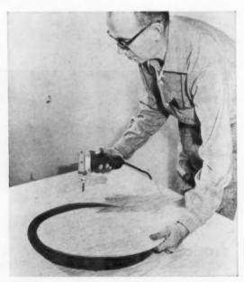
INSIDE CUT with Wen Model 505 sabre saw needs no starting hole. Air stream blows dust off guide line. Saw goes through wood or plaster, handles easily in overhead or vertical position. It is recommended for mounting attic and exhaust fans, radio speakers, and cabinet work. Circle No. 10010 on replay card, p. 134.
