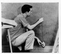
CHALK LINE by Evans, also used as plumb bob, has flush rewind handle; brake locks reel. Chalk refills through cap at plumb tip. Circle No. 10013 on reply card.
