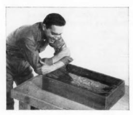
You can easily make this demonstration unit yourself! Just build a 24" x 12" frame out of 1" x 6" lumber. Staple 16" standard Balsam-Wool to the top, as shown. Fill with water—and for interest, add fish.
