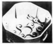
NEW PLASTIC OUTLET box by Porcelain Products, Inc., of Findlay, Ohio, is reinforced with molded glass fiber, has unusual resistance to moisture, fire and heavy impacts. It is noncorrosive and does not attract condensation, making it ideal for basement installation. Box is available with standard round knock-outs.
