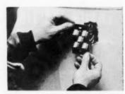
FIVE SWITCH CONTROL has standard size face plate which is screwed to plaster ring instead of a conventional box.
