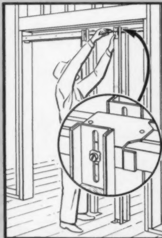
2. Install uprights After header is up, it's a simple matter to secure split jamb and split stud to header brackets.
