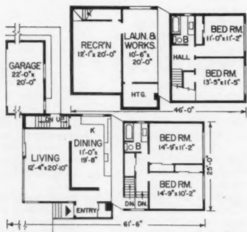
FOUR LEVELS of living characterize builder Quinn's Weldwood house. Recreation, utility level is under living level. There are two bedroom levels—one above the other.
