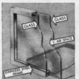
METAL EDGE. Ideal for large windows and where maximum insulation is needed most. Constructed of two panes of ½" clear-vision Plate Glass, with a ½" sealed air-space between. Exclusive stainless steel frame means no bare edges to chip or mar, as well as easier, quicker, and safer handling for the builder.
