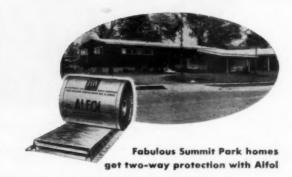
Close-up of Alfol blanket shows how award-winning Summit Park homes get full insulation plus a positive vapor barrier . . . all in one product. Multiple aluminum foil sheets space themselves automatically ... reflect radiant heat ... provide maximum year-round efficiency. Separate vapor-proof backing affords a positive and continuous vapor barrier . . . the finest protection obtainable against moisture condensation problems.
