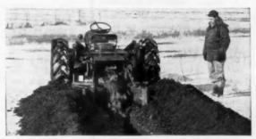
**Trencher digs up to 600 feet per hour,** 5 to 14 inches wide, as deep as 6 feet. Or, dig as deep as 13 feet, 12 to 24 inches wide, with heavy-duty backhoe.
