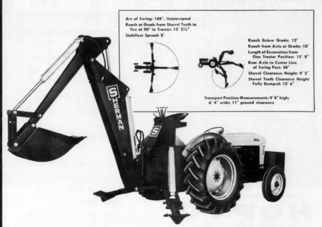
a few minutes by simply removing six pins and four bolts.
