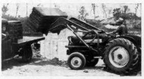
**Utility unlimited!** International 350 Utility gives 1,500-lb capacity with fork lift or half-yard bucket on the heavy-duty front-end loader... is easily equipped with rear-mounted fork lift.
