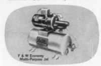
This economical jet pump converts from shallow to deep well by taking ejector off pump and moving it down into well. Substituting high pressure ejector enables higher discharge pressures, or use on deeper wells. ½ H.P. Motor, 480 G.P.H. & ½ H.P. 750 G.P.H. @ 15 ft. & 20 P.S.I. Available with 6, 12, or 30 gal. tanks.
