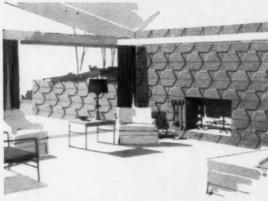
Shadowal block for the home adds new dimension and character to a room. The standard modular 8" x 16" face makes it easy to lay-up in the wall.
