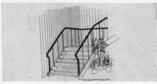
AN INTERESTING STAIRCASE design is achieved by applying vertical siding (thick edge to thick) over ½" plywood backing.
