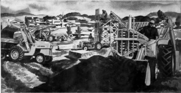
TYPICAL WORK BULL PACKAGES: Left foreground — 42-hp Davis Pit Bull with 7%-yd. loader. Left background — 34-hp Model 202 with 11 cu. ft. loader and rear-mounted backhoe that handles 12 to 36-in. buckets, digs to 12½-ft. depth. Center, Model 202 Fork Lift has standard 10-ft.
