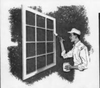
Prevent warpage in wooden components by back-painting with Aluminum House Paint: door frames, windows, sills.
