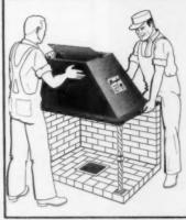
"Just set the Beneform on the brick, on two sides, and on corner post. Since Beneform has three straight sides, it's an easy matter to lay up brick. No lintel bars are necessary. Beneform's flange is 31/2" wide, strong enough to carry any load. Masonry is laid right on the flange. No fancy, time-consuming brick-work here."
