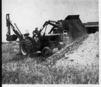
**FRONT-END LOADER** is the other part of the basic tractor rig. Scoop carries more than half a yard, can also be used to scrape and level loose dirt. Many builders use it to dump stone or slag into slab foundations.
