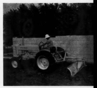
**BLADES OF MANY SIZES AND SHAPES** are available for both front- and rear-end mounting on tractors. This rear-mounted blade is designed for leveling and grading; its height can be controlled by the operator.
