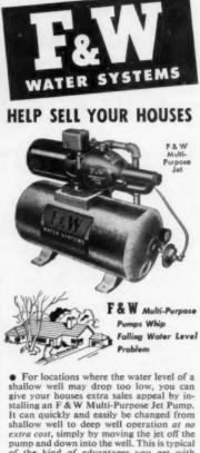
shallow well to deep well operation at no extra cost, simply by moving the jet off the pump and down into the well. This is typical of the kind of advantages you get with F & W Water Systems; whatever the re-quirements, there's an F & W Model to meet them exactly. All offer outstanding advantages in long life, dependable service, lowcost operation, and minimum maintenance.
