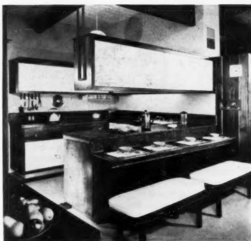
ALL-ELECTRIC kitchen is well-planned, has plenty of counter space and built-in appliances. Suspended cabinets are walnut-stained with sliding white masonite doors.
