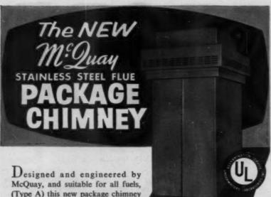
Designed and engineered by McQuay, and suitable for all fuels, (Type A) this new package chimney has a 7" stainless steel flue with aluminized steel interliner and outer casing. The interliner is supported by the exclusive McQuay stainless steel tension spring spacers for strength, rigidity and durability.
