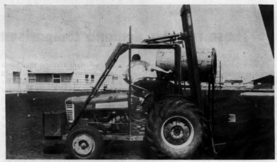
FORK LIFT attachment can be a permanent installation, like this one, or an additional attachment for the frontend loader. Though not an actual earth-moving item, it is a valuable bonus that goes with the small tractor.
