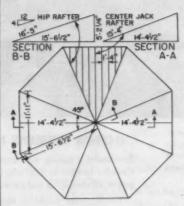
ANSWER: In the above diagram you'll find all of the data needed to lay out your proposed octagonal roof. The sectional view A-A gives the dimensions for the center jack cuts. B-B shows dimensions for all of the hip rafter cuts.
