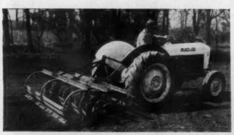
PREPARATION of ground for final seeding is done quickly with this attachment, that rakes, breaks up dirt clumps, and finally combs the ground out smoothly.
