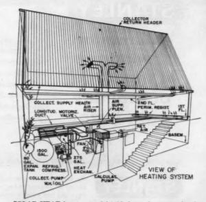
SOLAR HEAT is augmented in this house by conventional oil-fired hot-water system to cover long span of sunless days.
