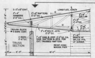
TRUSSED RAFTER section (above), roof framing plan (right) illustrate how the unusual roof is constructed. Though the diamond-shaped roof looks complicated to build, experienced carpenters had little trouble framing it. Architect: Duane Conner, Oklahoma City.
