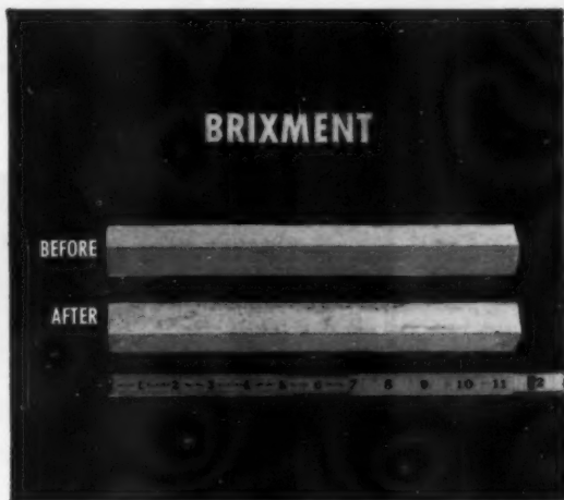
In these autoclave tests, neat cement bars were exposed to 295 lbs. steam pressure, 420°F., for 3 hours. Left: The two bars are both Brixment. Note that it is sound—it has not
