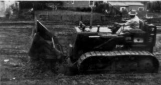
**He can roll the earth** with the 4-in-1's big capacity bulldozer action—obtained by lifting the 4-in-1's clam lip hydraulically and regulating depth of cut by radius control. There's blade curvature for live dirt action; strength for hard dozing.
