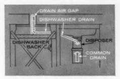
Sanitary Drain Air Gap—Eliminates need for prior roughing in, provides maximum sanitation, uses one drain for both dishwasher and sink. (Optional: sanitary drain which utilizes existing sink.)
