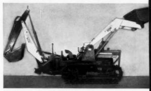
New International T-340 delivers 45 gross engine hp. Shown above with International Wagner backhoe and loader, the T-340 can be equipped with Torque Amplifier Drive or Fast-Reverser unit.
