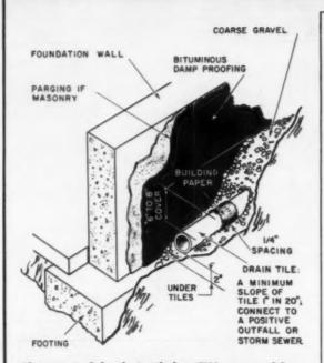
Placement of the drain tile has FHA approval for minimum acceptable protection. For maximum protection, tile should be laid on the same plane as footing. Joint between foundation and footing should be flashed.
