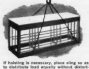
Check to make sure window is perfectly square; transit damage may have caused misalignment.
