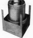
Starter Box and Starter Section in one unit for fast erection. Interliner and stainless steel flue supported by exclusive McGuay stainless steel and aluminized steel tension spring spacers. Permits quick drafts and even temperature top to bottom for peak efficiency under steady or intermittent firing.
