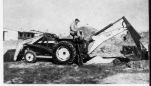
Three 6-cylinder power ratings, 61 to 90 gross engine hp all available with gasoline, Diesel or LP Gas engines. Above, the 61 hp International 460 Utility with International Wagner backhoe and loader.
