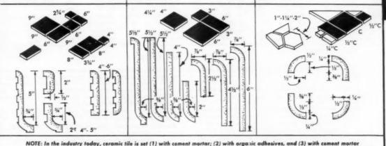
NOTE: In the industry today, ceramic tile is set (1) with cement mortar; (2) with organic adhesives, and (3) with cement mortar --using a newly-developed thin-setting bed method. Information on all three methods may be obtained from the Tile Council of America, Inc., 800 Second Ave., New York 17, N. Y. Courtesy Tile Council of America
