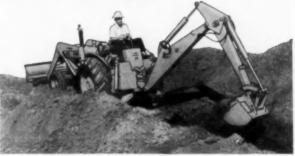
The center-mounted John Deere 50 Backhoe has 205-degree boom swing. In tight spots, digs at 90-degree angles to tractor.
