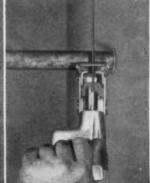
BLADE LIFE DOUBLED. Shoe can be repositioned easily with screw driver to use new cutting area of blade after one part is worn. Actually doubles blade life.
