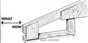
shows how Stream builds his cornice framing directly onto each truss. Soffit is formed by a horizontal 2x2 and a vertical 2x4 which are stapled and glued to the outlooker on the end of the truss.
