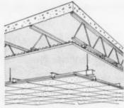
THIN CONCRETE FLOOR is shielded by intermediate plaster ceiling suspended beneath it.
