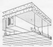
IN STRUCTURAL STEEL SYS-TEMS, insulating material is sprayed on undersides of members.
