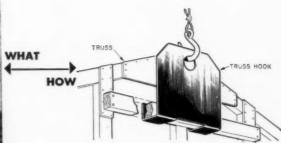
crane and benefit from the construction speed it makes possible. It enables Stream to put up a truss a minute with a six-man crew. Drawing shows the special fitting used to lift trusses and gable ends.
