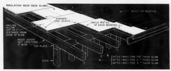
Rafters should be at least 3 in. nominal width. Maximum spacing of framing members should be set at 16 times slab thickness. Thus, 3-in. thick decking permits beam spacing
