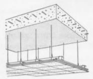
REINFORCED CONCRETE is protected by suspending acoustical ceiling from the slab with metal hangers.
