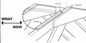
stead of joining several trusses with long 1x3 ribbons, his crews attach a scab to each truss with a single nail. When the truss is installed, the scab is pivoted out and nailed to the preceding truss.
