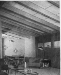
Ideal for modern exposed-beam construction, this one product combines roof deck, insulation, sound-quieting, finished ceiling and continuous vapor barrier. <u>VAPOR SEAL TYPE: 2' x 8' in 2" and 3" thicknesses</u>. STANDARD TYPE: 2' x 8' in 1½", 2" and 3" thicknesses.
