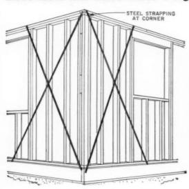
Cost of corner bracing is reduced by using steel strapping instead of let-in wooden braces. Straps are nailed up in an "X" pattern as shown. Stream estimates a saving of 20 minutes at each corner.
