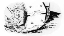
hand shovels. To boost traction of the machine's treads in frozen or muddy ground, Stream puts two 1-in. diameter bolts into each tread section. The bolts are secured with locknuts, as shown above.
