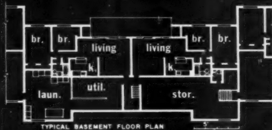
GROUND FLOOR BLOCK has either one utility area, as here, or two, in the case of a middle unit.
