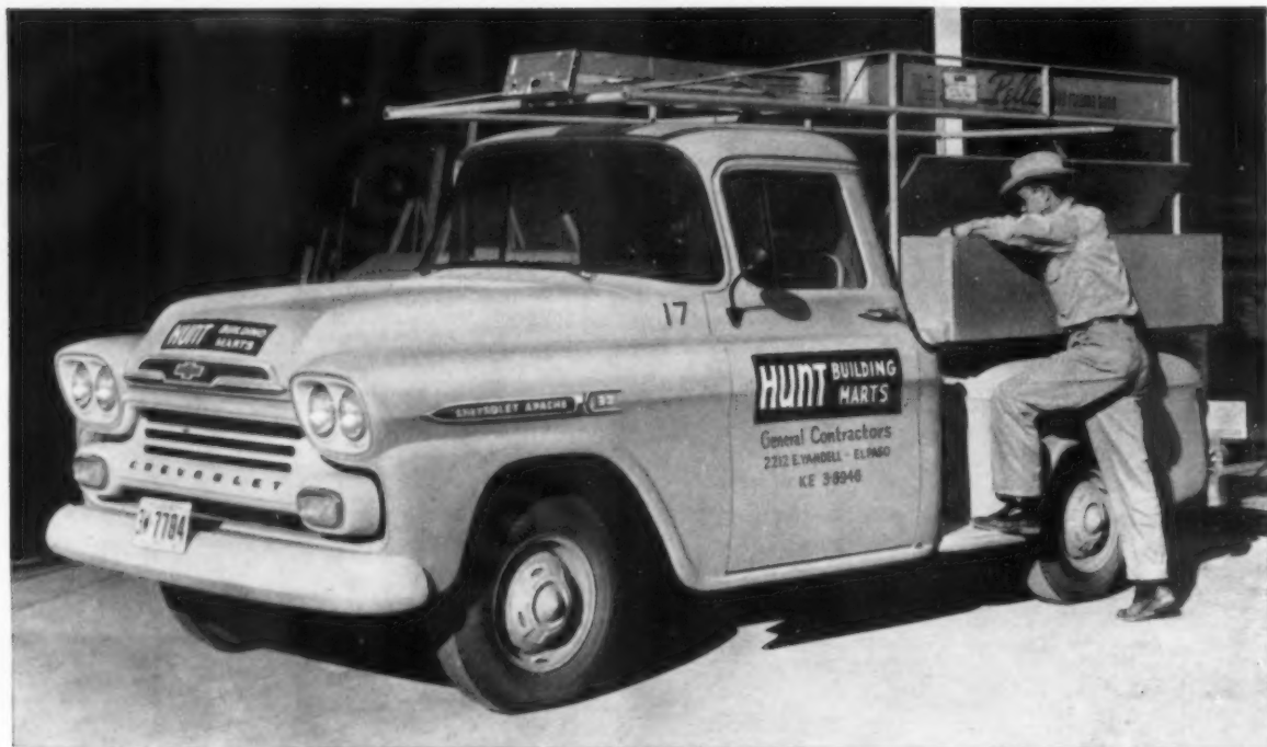
SEVEN HANDY STEPSIDE MODELS, with side running board, provide spacious bodies in 78", 98" and 108" lengths. As shown above, both Stepside and Fleetside models can be easily equipped to handle special work needs.
