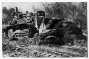
New International Drott T-340 Four-In-One Skid-Shovel—combines in one machine a bulldozer, clamshell, carry-type scraper, and ¾ cu yd bucket (% cu yd heaped), all hydraulically controlled.
