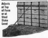
Newest addition to Symons line . . . steel form brace. It is easily tied to pre-fab or built-up forms and to wooden or steel stakes. Once attached, brace can be adjusted at top of form or at stake level for positive alignment. Comes in regular lengths of 6' and 10'6". Brace extensions available.
