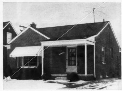
IF THIS HOUSE were like the story-and-a-half next door (at left), expanding into the attic would present no problem. The roof could be swung up on one side of the ridge. But on the house with the low ridge line, the whole roof would have to be raised. However . . .
