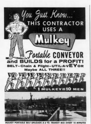
Concrete, sand and gravel may be delivered directly from truck to gravity hopper without intermediate handling, maintaining a continuous flow of materials from truck to point of use on the job.
