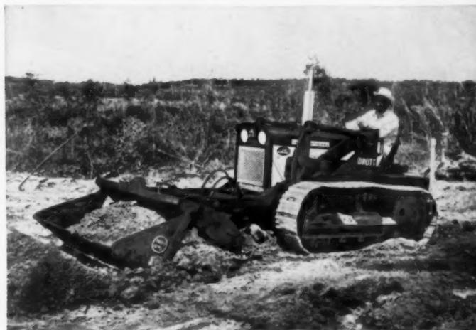
**It's a clamshell** with exclusive ability to "surround" loose materials for loading, and to dump sticky materials through the bottom of the bucket.
