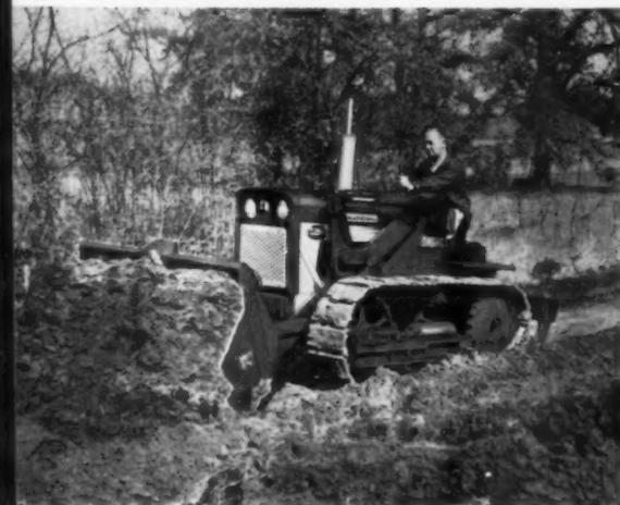
**It's a Skid-Shovel** with patented pry-over-shoe break-out action which gives over 5½ tons of break-out force, for prying out stubborn materials, stumps, and boulders.
