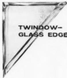
**TWINDOW—GLASS EDGE.** This type is just the thing for modern window-wall construction. Having exceptional insulating properties, it is constructed of two panes of 1/4" PENNVERNON®—the quality window glass—with a 1/2" air space between. TWINDOW—glass edge units are available in popular sizes for a variety of window styles.
