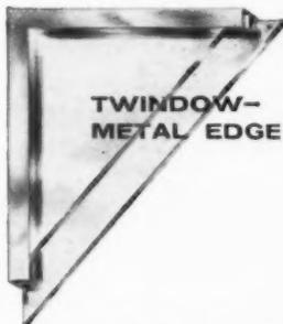
**TWINDOW—METAL EDGE.** This type is ideal for large windows and where maximum insulation is needed. It's made up of two panes of 1/4" clear-visibility Plate Glass, with a 1/2" sealed air space between. Its stainless steel frame, a TWINDOW feature, eliminates bare edges . . . makes handling safe, quick and easy.
