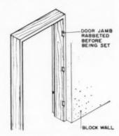
Here's how we avoid a big headache in block, and other masonry construction: before installing door jambs, we rabbet them to take the door hinges. With this system we eliminate any possibility of having the jambs come loose, as often happens, when they're rabbeted in place.
