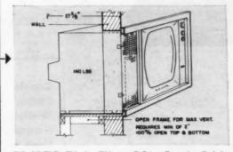
TO BUILD IN the TV set, RCA offers detailed installation drawings. Sets are 43, 81, or 140 lbs.
