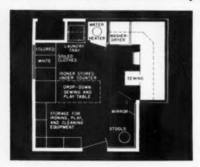
THE COMPLETE utility-work room includes a high percentage of laundry area. This plan lines up water heater, washer-dryer, cabinets and counter, allows a sewing machine nearby. Laundry tray, hampers and ironer fill out other side of the "U." Design, by American Home Magazine, is a step-saving layout.
