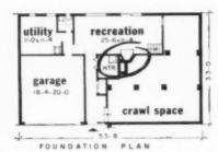
By combining two fireplaces and a furnace in a central location, brother-builders Ralph and Sid Paul can run three flues up a single chimney. They estimate the over-all cost savings at \$450 to \$500 per house.
