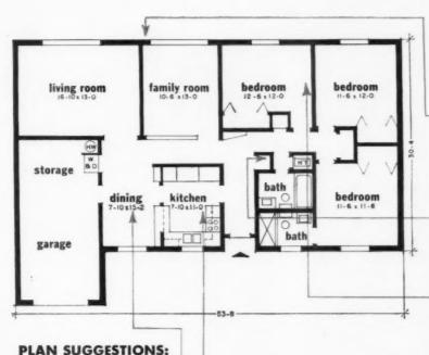
"Arrange kitchen equipment in 'U' shape and screen from dining area. Room divider could be some form of pass-through. Countertop 3' above floor could serve as a snack bar. Shelves behind cupboard doors for china are well-located: table can be set from dining area, washed and put back on shelves which are close to kitchen sink.
