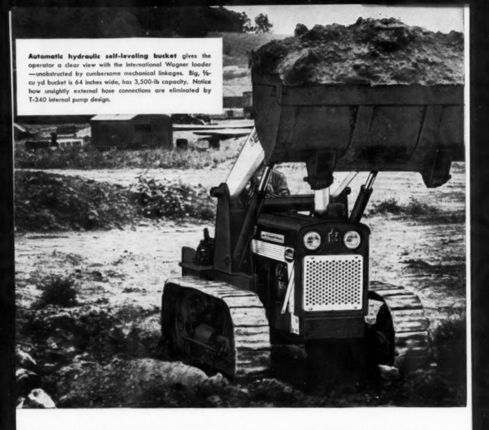
New International Drott Four-in-One. Only the new T-340 offers this versatile, high-production unit in the utility crawler field! Left below, showing exclusive clamshell action for "surrounding" materials, or dozing close to green foundations without excessive ground pressure. Right, bottom-dump action provides 9 ft, 6-inch
