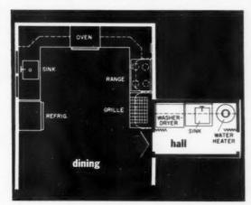
ANOTHER COMPACT COMBINATION . . . this time in a hall closet with folding door for screening. Here, the laundry area is on its own, out of the kitchen, but still near enough to keep the two work areas handy. Sink separates washer-dryer and water heater; storage tops all three units. A Living for Young Homemakers kitchen.
