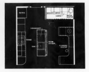
THE LARGER KITCHEN, or the smaller one, can easily use this laundry arrangement (red area on plan above). Washer, dryer (or combination), cleaning cabinet, and water heater can be arranged compactly. Cabinets above and folding curtain door complete this "hidden kitchen value." By Hallmark Kitchens.
