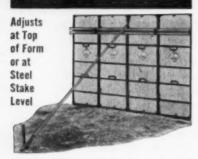
Newest addition to Symons line . . . steel form brace. It is easily tied to pre-fab or built-up forms and to wooden or steel stakes. Once attached, brace can be adjusted at top of form or at stake level for positive alignment. Comes in regular lengths of 6' and 10'6". Brace extensions available.
