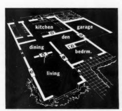
FLOOR PLAN gives six suggestions for location of Mural TV set. All styles have controls and speakers in front. Ventilation louvers can go in front or receiver be vented from the back.
