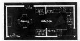
**SMALL KITCHEN** packs a lot of service in a minimum of space. Unbroken counter space is achieved by centering sink, putting range and refrigerator at extreme ends of the "U."—American Home Magazine.
