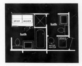
THROUGH THE MIRROR you can see the washer and dryer in this bath. They face the sink and toilet, are closed off with a folding door. Laundry storage units are above the machines. Plan puts laundry into both bath and cleaning centers, (see plan). Keeps it handy to bedrooms, too. Built by Mannon Associates, Denver.
