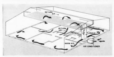
RADIAL DUCTWORK was eliminated from this warm-air system. (NAHB Research House). Furnace is on top of perimeter duct, near exterior wall.
