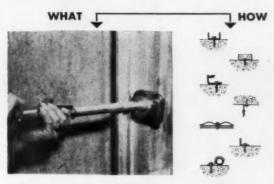
APPLICATIONS UNLIMITED . . . Powder-actuated "Drive-It" nails almost anything onto concrete or steel.
