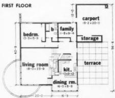
FLOOR LAYOUT will fit the needs of either the small or large family. The first floor has all of the necessary rooms for a family of two: sleeping, working, dining, and living.
