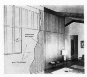
Plywood shear walls eliminate bracing on all other walls and permit use of large glass areas on the view side. Used in pairs (see floor plan), they work with the horizontal plywood floor and roof diaphragms in resisting high wind or earthquake loads. At least one shear wall on every home is continuous from foundation to roof.
