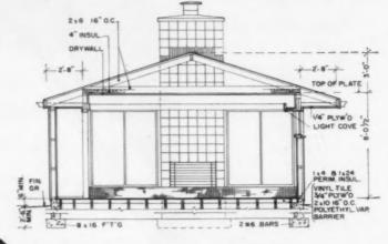
HOUSE SECTION shows the 56-in.wide chimney, plus tiled window seat and hearth in front of it.
