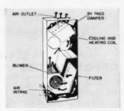
A LOOK INSIDE. This Arkla-Servel unit has simple operation. Works on absorption-refrigeration principle.
