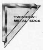
TWINDOW—METAL EDGE. This type is ideal for large windows and where maximum insulation is needed. It's made up of two panes of ½" clear-vision Plate Glass, with a ½" sealed air space between. Its stainless steel frame, a TWINDOW feature, eliminates bare edges... makes handling safe, quick and easy.
