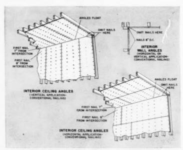
"FLOATING" Gypsum wallboard in wall and ceiling angles reduces board stress. Elimination of nails does it. Gypsum Assn. (No. 082, p. 166)
