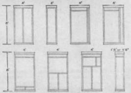
8 basic panels are used, with %" PlyScord® sheathing over  $2 \times 4s$ , 24" o.c. Window frames are installed by fabricator. Sections rest on %" fir plywood sole plate and are tied together by a continuous couble  $2 \times 6$  header.
