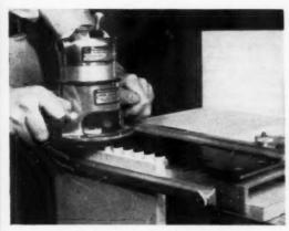
A real selling extra for home builders—dovetailed drawer joints. Quickly and accurately cut with Porter-Cable Router and precision Dovetail Templet.
