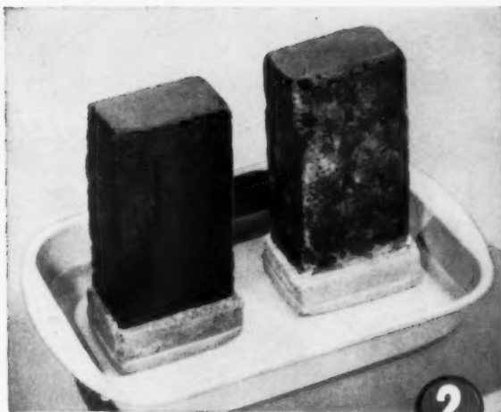
2 Keep about 1/2" of water in the pan for at least one week. Even if soluble salts are present in the brick or sand, you will soon be convinced that Brixment mortar helps prevent efflorescence.
