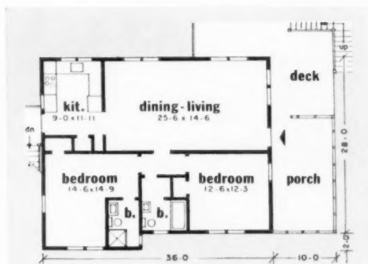
FLOOR PLAN , as simple as the elevation, stresses living space—both inside and out. For year-round comfort, the house is equipped with electric water heater and refrigerator, gas range and furnace.
