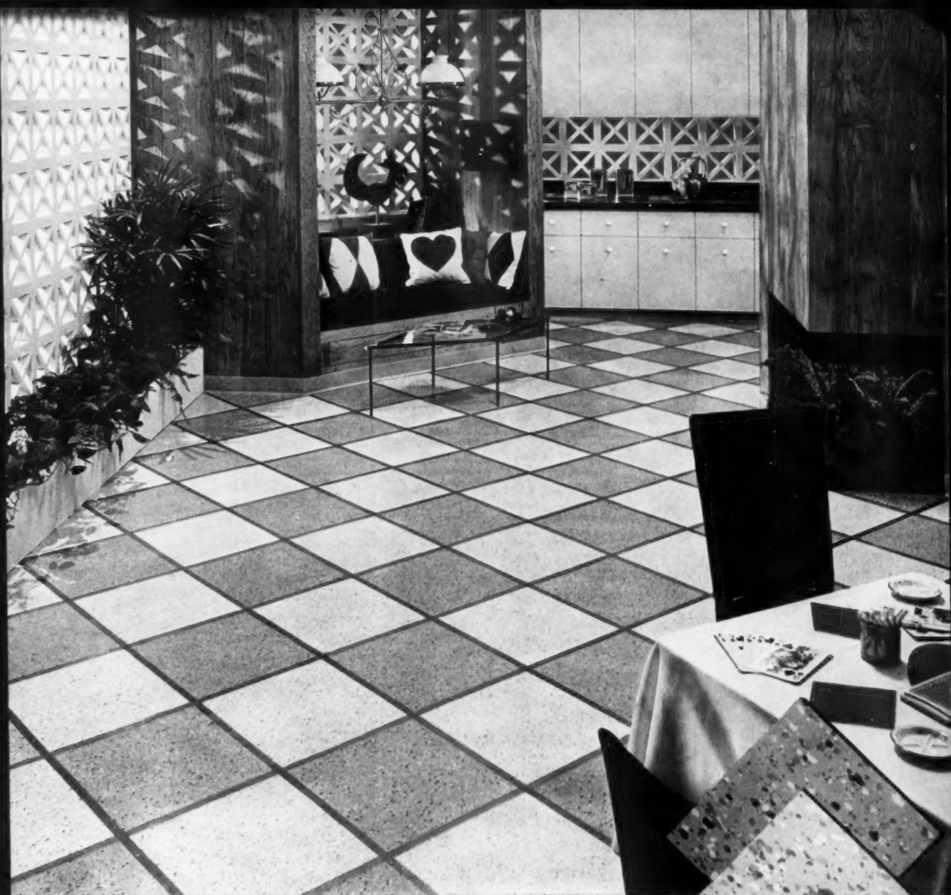
Rooms above feature Metallic Style Kentile Vinyl Asbestos Tile in Autumn Gold and Dawn Gold, with Gold Feature Strips. Wall Base is Beige KenCove.
