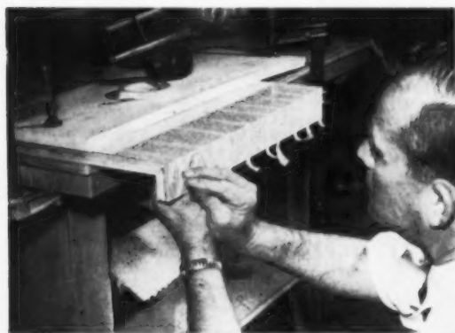
STEP THREE —A few strips of cellophane tape keep the bevels firmly in place until the waterproof glue dries.
