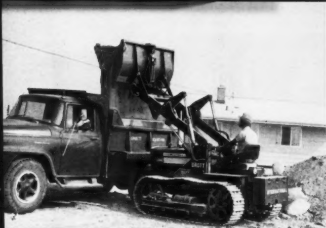
Dumping through the bottom of the bucket clears sticky materials, increases dumping height to 9 ft, 6 in.
