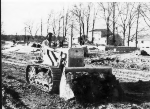
In scraper position the 4-in-1 loads from the bottom with the fast, live "boiling action" of earthmoving scrapers.
