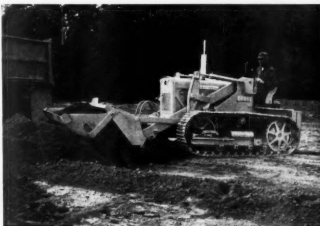
With the 4-in-1 clamshell you have exclusive ability to "surround" loose materials instead of chasing them.
