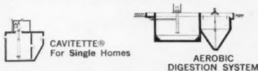
ACTIVATED SLUDGE PROCESS
