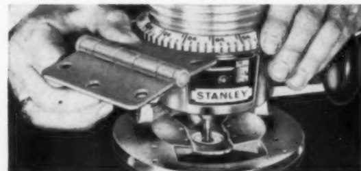
PRECISION cutting is feature of router's micrometer depth adjustment which permits very accurate setting.
