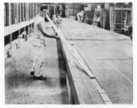
**3** Pattern strips are inserted into grooves running length of table. When house will be repeated, strips have cleats—to form slots into which framing members fit exactly.
