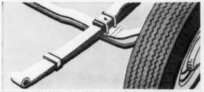
SAVE UP TO \$150 ON FRONT TIRES! In certified tests of truck suspensions, Ford front tires lasted up to twice as long. In 50,000 miles savings can add up to \$150 on a pickup... more on two-tonners. And Ford's sturdy I-Beam front axle and leaf-spring suspension not only cut tire wear, but their simpler design also cuts maintenance costs.
