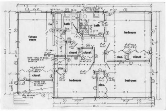
**1** Exterior and interior walls are divided into segments that can be easily handled and transported, generally weighing less than 350 pounds each. Walls will be assembled in a continuous strip on a 175 foot long table . . . then disassembled into segments as planned. Segments are numbered both on plan and on executed wall sections for orderly assembly at site.
