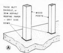
By taking just a little extra care you can greatly increase the life of wood posts and timbers that come into direct contact with masonry.
