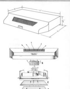
Powerful fan (A) draws odor and grease-laden air through the Grease Filter (B) and the Activated Charcoal Filter (C), then recirculates pure fresh air through grille at top.
