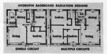
FOR MAXIMUM ECONOMY, arrange baseboard in series, using single circuit in installation of less than 35 MBH: multiple circuits for larger loads.
