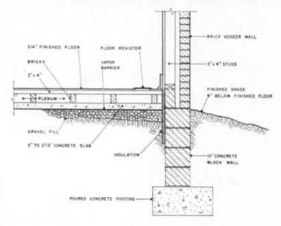
A type of heating system that's getting more attention from builders is one in which space between the wood floor and concrete slab acts as a warmair plenum.
