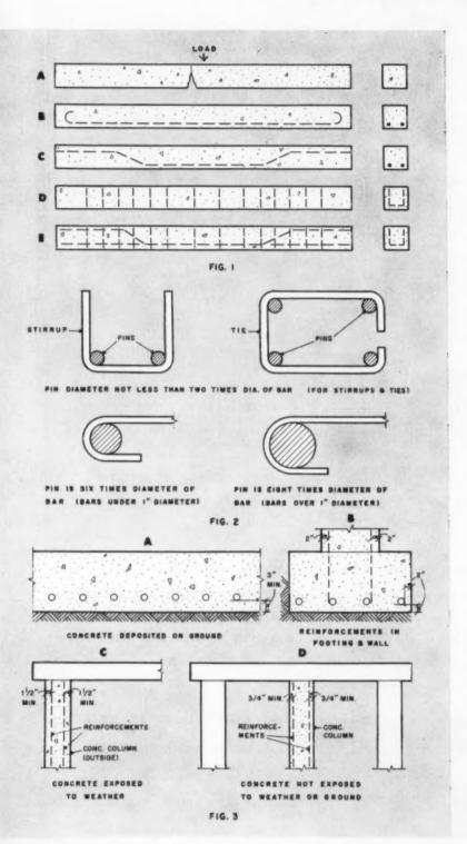
**C**ONCRETE is strong in compressures and loads. However, it's comparatively weak in resisting pull or tension. Therefore, reinforcements-round or square steel bars, or mesh-are used to increase its tensile strength.
