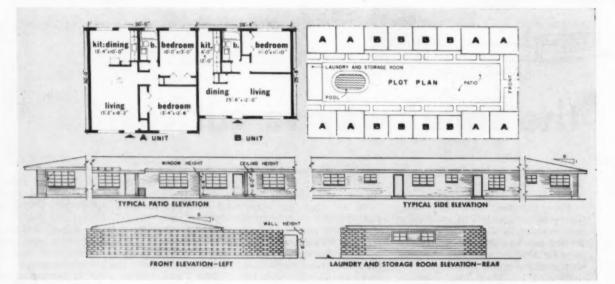
PLOT PLAN shows clever grouping of apartment units around pool. Lot size is 157x298.6'. Street side is enclosed by an 8' deco-
