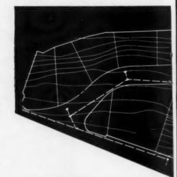
below a series of artificial terraces run parallel to both. Five in all, the terraces were cut by a bulldozer in a consecutive slope, flat, slope, flat sequence.
