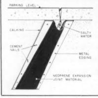
Parking garages during the winter months are often faced with the problem of salty water running off parked cars and dripping down through floor cracks onto cars below. Calking doesn't stop drips.
