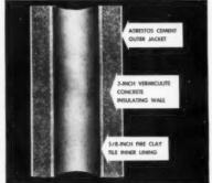
The fire-clay tile liner of the Van-Packer chimney won't corrode. It outlasts other factory-built chimney flues, and provides more efficient service because it retains heat longer for better draft. Fire clay is acidproof, withstands temperatures up to 2100°F, and won't dent, flake or corrode even under severe conditions.
