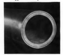
Made of 5%" fire clay tile with a corrosion-resistant jacket, this gas vent is acidproof, fireproof, and won't dent, rattle, corrode or flake off. It is UL-listed for Class B service, for all gas-fired appliances (except incinerators) requiring a 3" to 7" ID flue. Model G gas vents are available with Van-Packer asbestos-cement or metal housing, or with kit containing flashing, storm collar, and rain cap.
