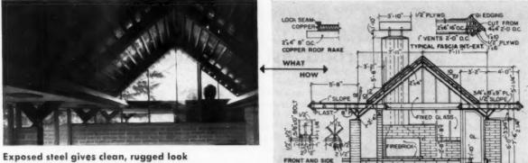
Concrete block walls combine with steel roof framing and glass walls to enclose modern living room. Extended soffit, held in steel elbow of gable, floats in space above glass wall.
