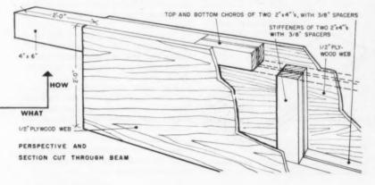
Use of the box beam, Kinney says, meant the house was under cover in record time. It also allowed the entire second floor to be free of bearing partitions for a completely free design.
