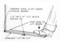
Barrel staves to lift gypsum wall-board in place (AB, June, '61) are hard to come by in Chicago, reports Paul Mandaback. A good substitute is a scrap of 1x3 or 1x4 with a 1x2 or 2x2 tilt block nailed on, as shown left.
