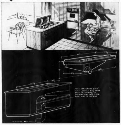
Work with existing ducts or with a unique downwardflow system that eliminates hood, cuts installation costs
