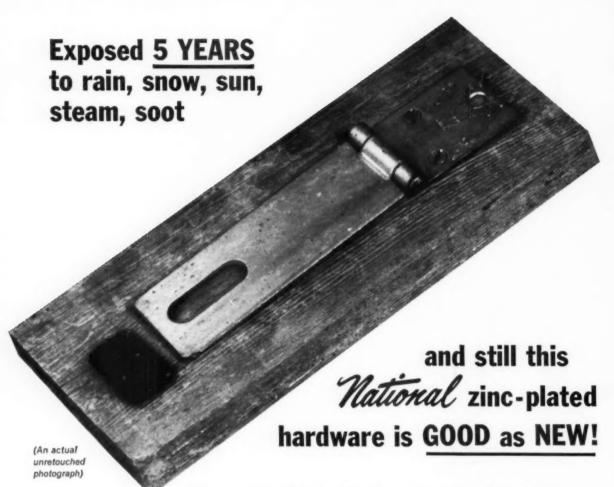
This weathered board with safety hasp remained for 5 years on the boiler room roof of the National factory. The hardware was exposed to rain, snow, ice—all the elements—plus soot and steam from the boiler room. Notice how the National zinc-plated hasp came through this grueling test with no trace of rust.
