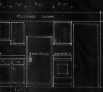
KITCHEN ELEVATIONS SCALE 3/16" = 1'-0"
