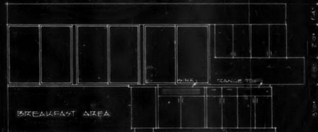
ELEVATION 2 KITCHEN ELEVATIONS SCALE 3/16" = 1'-0"
