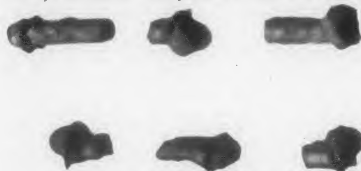
Fig. 2. Showing Rivets Defective for Various Reasons; Also Burned Rivet Before Driving
