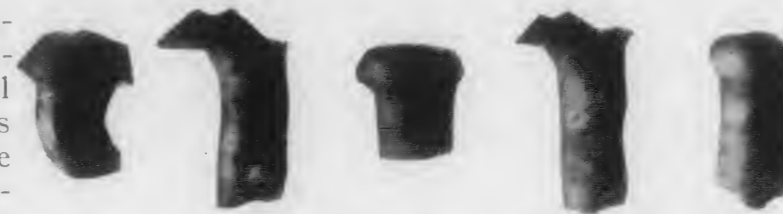
Fig. 1. Showing Rivets Driven "Too Short", Also Heads Not Concentric With the Holes
