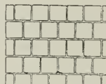
When square tiles are laid with broken joints, long lines in one direction are the result.
