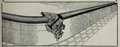
SECTIONAL VIEW OF DOLBEAR CURB BAR IN CONCRETE
