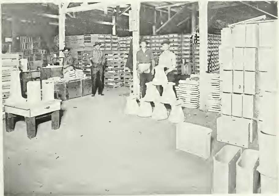
Warehouse. Pieces are here given final inspection. Assembling and fitting of brass parts is done, and stock is piled for shipment.
