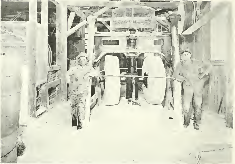
The grinding stones. This is the first step in the pulverization of the material
