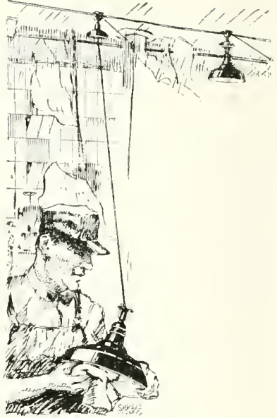
Cut-out and Lowering Device for Electric Light Fixtures
