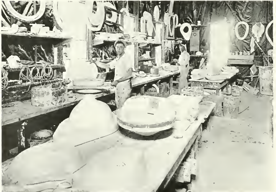
The mold shop. Plaster models and molds are made in this shop.
