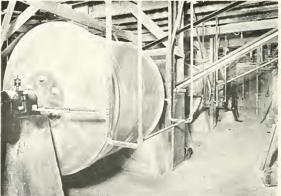
The ball mill. Rotating cylinders containing balls which pulverize the material to a fine powder.
