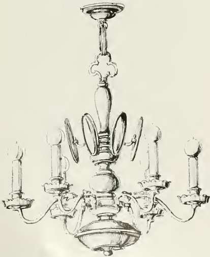
A pewter ceiling fixture with polished metal reflectors. Designed for Mr. J. S. McClymont. Albert Farr, Architect . J. Francis Ward, Associate .
