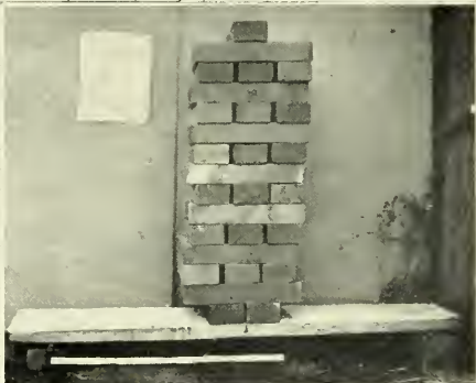
Slab No. 21. 1 1/2" x 12" (no reinforcing) Span 40", Central load 295#. Ult. L. = 321# M = 1/8 lbd 2 = 3210 + 300 (for slab wt.) = 3510# Modulus of Rupture = M ÷ bd 3/16 = 1,120 #/sq. Note that the specimens reported above were allowed to set and were cured without restraint (other than that provided by form friction and by the bars in specimen No. 23) Fractures of 21, 22, & 23 showed aggregate pulled apart on tension side of slabs; even small particles of hard gravel.
