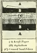
Sisalkraft is composed of crassed layers of sisal fibres imbedded in asphaltum and covered by layers of heavy kraft paper. The construction is exclusive. Made in rolls 3, 4, 5, 6 and 7 feet wide.
