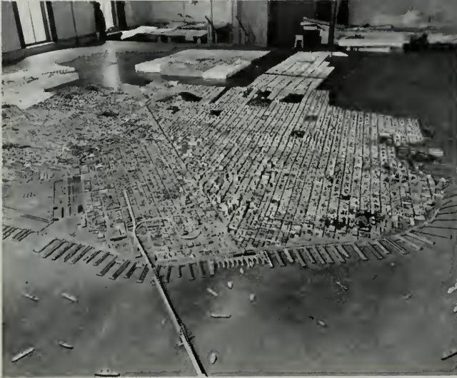
Scale model map of City of San Francisco, mounted on platform, 41 x 37 feet and built to scale of 1 inch to 100 feet.
