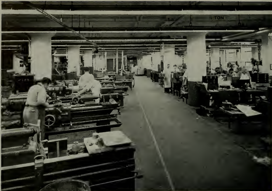
Visibility and lighting efficiency are greatly enhanced by the white ceiling and columns in the machine shop shown here.
