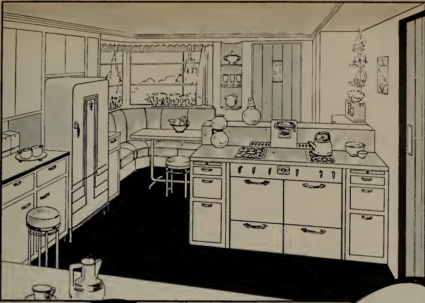
A modern kitchen, designed by a member Gas Company's Planning Department, showing step-saving arrangement of work centers and correct placement of appliances.
