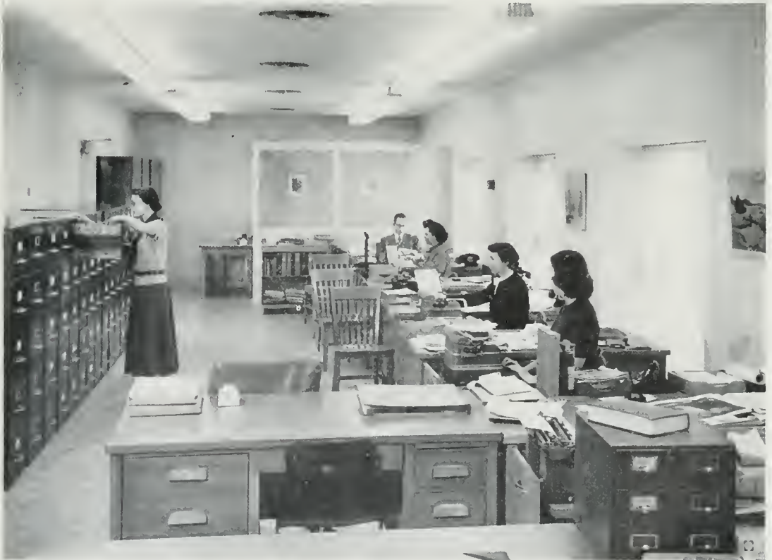
ONE of the smaller departmental general offices in the new annex—combination day-lighting and indirect electrical lighting provides ample light while floor and ceiling construction minimize noise.
