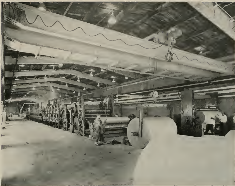
LOOKING down production line of paper-making machines—side walls and roof strongly reinforced for large overhead crane.
