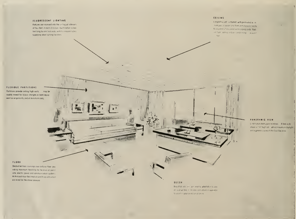
SKETCH of typical office with fluorescent lighting, completely self contained ceiling, flexible partitions providing ceiling high walls, decorative floor covering over cellular floor with four foot module system for location of partitions, electric power, communications systems.
