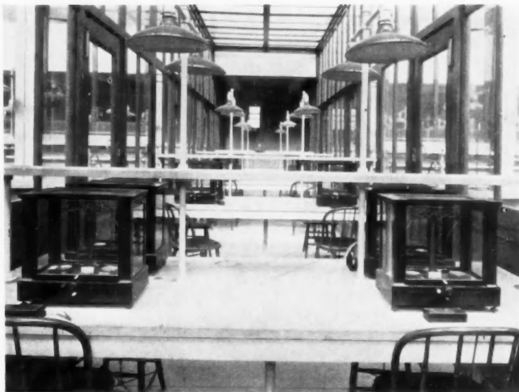
Because of the extremely delicate types of instruments housed in this balance room at Sterling Chemistry Laboratory, the room is ventilated only by air forced in. It is exhausted only when the doors are opened
