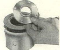
The Flat Plug is removed from cover and the cover is reversed. Note the high rim protection on "in service" side of cover
