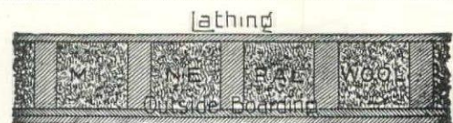
Section of Outside Wall of House, Showing Wool Between Studding
