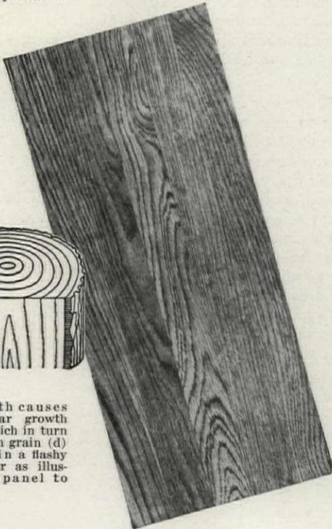
Slow growth dependent on ideal climate soil and drainage in the Appalachian Highlands causes narrow annular growth rings (a) which in turn produce close grain (b) resulting in a fine grained floor as shown in panel to right.
