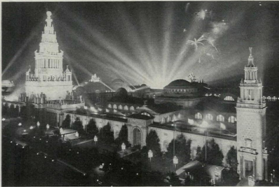
Night view of the Tower of Jewels and Manufacturers' Building, Panama-Pacific International Exposition. This illustrates the preservation of depth, or the third dimension in light, by a combination of white floodlights and colored relief light.
