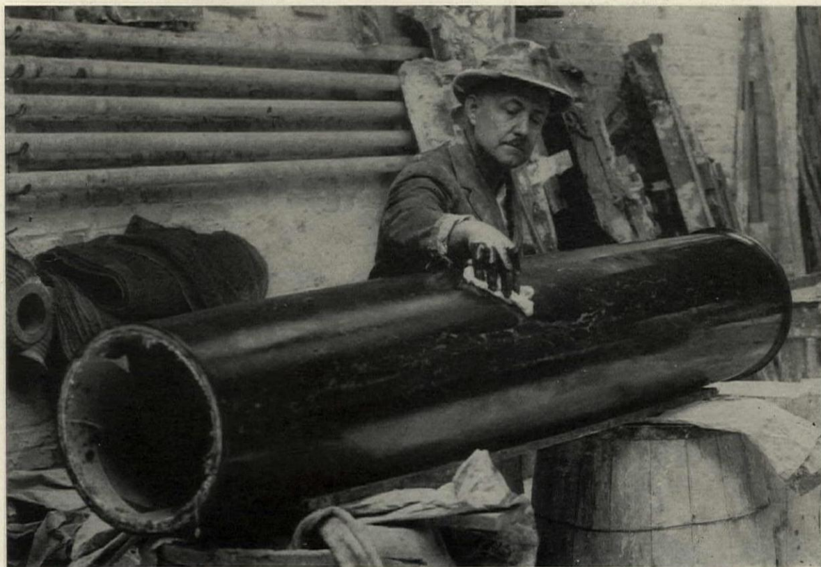
A Small Black and Gold Column of Artificial Marble Being Polished in the Shop
