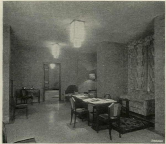
Writing Room with Modern Fixtures for General Lighting. Ceiling Fixtures have 100-Watt Lamps
