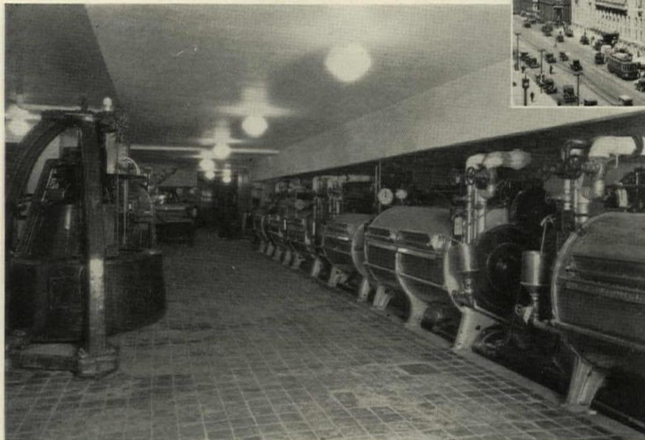
The Royal York Hotel, Toronto, Ontario, Canada, owned and operated by the Canadian Pacific Railway Company, with a view of the monel metal Cascade Washers and Humatic Extractors in its indispensable laundry. This airy, well-lighted department was designed in collaboration with the engineers of The Canadian Laundry Machinery Company. Ross & Macdonald, Architects; Anglin-Norcross, General Contractors.
