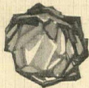
Microscopic drawing of a grain of quarried sand. Note its rough surface—its many angles and faces. Such a grain of sand has a larger surface area than a round, smooth grain. Consequently, it will be attacked much quicker by the flux and the batch will melt much faster.
