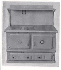
HEATERANGE. The Jeddo Highland Heaterange, to all appearances a coal burning cooking stove, is also a warm air furnace from which, by the usual arrangement of ducts, blower, and humidifier, warm humidified air is circulated throughout the house. As with other furnaces, a water back and storage tank provide for the supply of domestic hot water.
