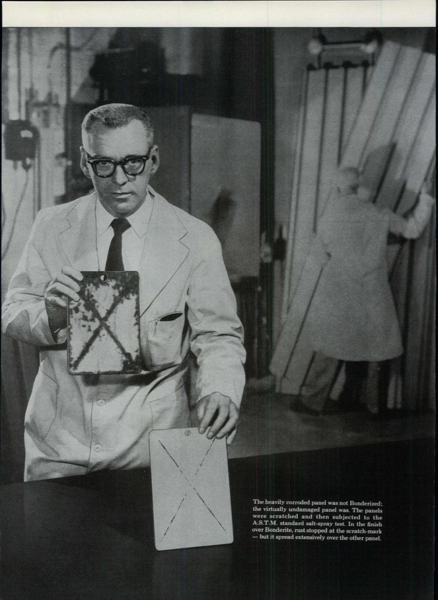
Continuous 8-day salt-spray test proves prime advantage of Milcor steel roof deck
