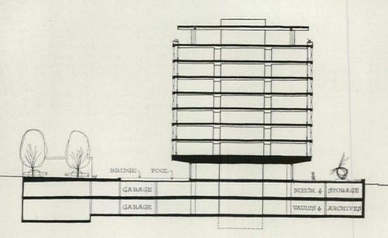
Section through building shows parking garage and vaults below the pool. Loss of usable space per floor (owing to the double wall system) is about 1,000 sq. ft., but building cost is same as a standard wall system.
