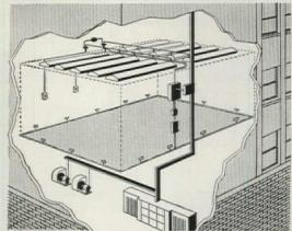
CUTAWAY shows basic loads—lighting, motors, general service—supplied by G-E 480Y/277-v equipment with fewer feeders, components than 208-volt system. Result: savings in space, equipment costs.
