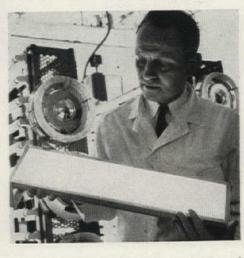
rescent light. The new lamp is composed of a labyrinth or maze of passages sandwiched between glass sheets. Thus the arc or electrical discharge, instead of traveling in a straight line as in the conventional tube-type fluorescent lamp, travels through a winding path to produce an area (rather than a line) of light. The model shown above measures 8 by 12 in., and only 1 in. thick—a factor which will reduce the amount of ceiling space needed for overhead lighting installations.
