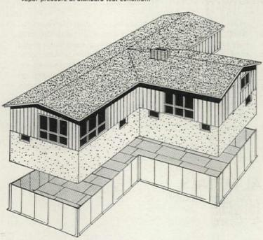
COMPARE the strength . . . "PREMOULDED MEMBRANE" is strong enough to maintain its permeance rating after it has been subjected to the pouring of aggregate, trundling of wheelbarrows and installation foot traffic. Resists rupturing and tearing. How many other materials will perform like this under the above circumstances?
