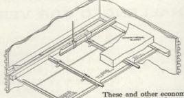
This isometric drawing shows all 4 parts assembled — a relatively simple construction that replaces the conventional radiators, or hot air ducts used for convectional type heating, and that permits reduction in size of air handling equipment such as blowers, fans, coils, filters, etc.
