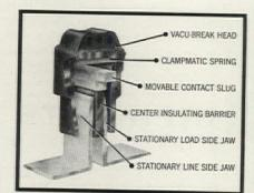
Close-up of Vacu-Break head shows movable contact slug inside the compact arc chamber. The Clampmatic spring assembly assures a bolt-tight contact, helps speed "break". This combination guarantees positive and safe operation, long switch life.
