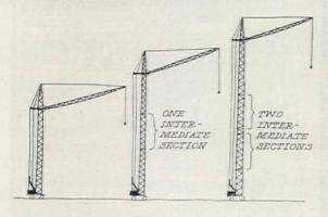
Tall German crane, with 153 ft. tower and 70 ft. jib, sets a form for a concrete end wall on this 12-story parking garage in Boston, being erected by Wexler Construction Co. As sketches (left) show, the height of some models can be extended to maximum of 300 ft. by the addition of intermediate sections. Reach of the jib is governed by crane height and weight of the lead; maximum jib length is 127 ft.
