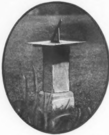
For accuracy a sundial must be set to fit its actual location at exact noon in late December or June
