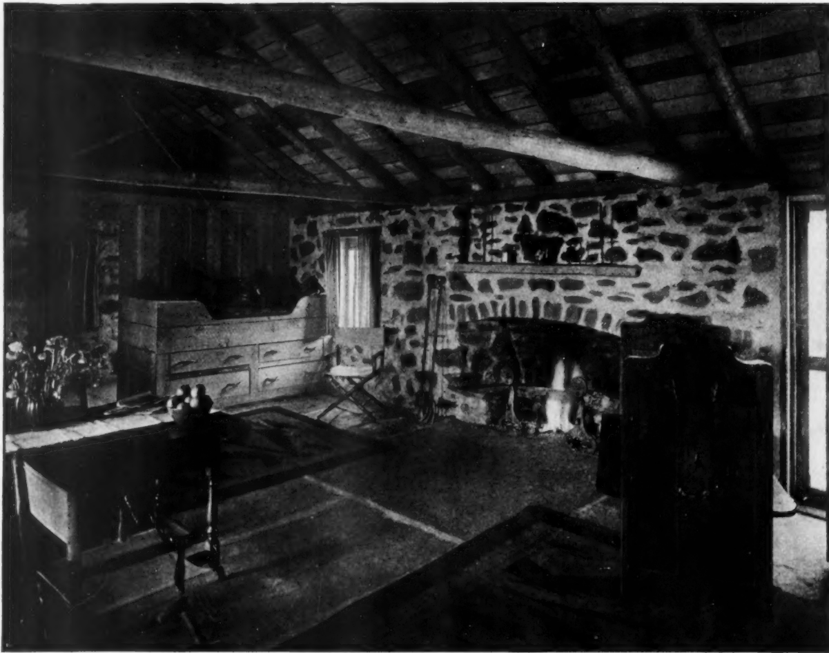
A wide rough-finished fireplace, high built-in beds, and a double reversible fire bench are the salient features of the living-room, which runs the entire width of the cottage. The floor is of flagging
