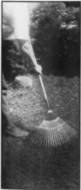
A modern lawn broom that really is a rake with pliable prongs. It sweeps clippings and refuse
