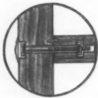
To facilitate setting up and dismantling, and to insure rigidity in use, Stickley beds employ the rail and post assembly shown in the cross-sectional drawing above.
