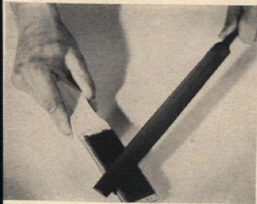
Keep your wood and metal files in top working order by keeping them clean. You can do this easily with a "file card" (a flat brush with short, stiff bristles). Stroke card across file grooves to remove residue after each filing job.
