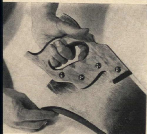
You can prevent the teeth of your hand saws from becoming dull and bent with this simple device. Cut a piece of rubber tubing the same length as the saw blade and split it down the side with a knife. Then slip tubing over the saw teeth. This is an excellent precautionary measure to take whether or not you have a wall rack for saws in workshop.
