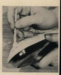
Touching up nicks and chips in the paint on refrigerator, furniture and woodwork is a big chore when you have to clean the brush after such a small job. Try a pipe cleaner, bent over and twisted as shown. It does an excellent touch-up job.
