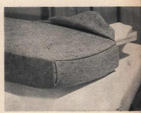
11. Brush coat of glue on back between braces; cover with cotton batting equal to thickness of braces. Pull fabric up and over pad. Fold corners. Trim, tuck in and stitch sides at back edge. Screw back to seat with angle brackets. Fold fabric under seat, pull taut, tack, press.
